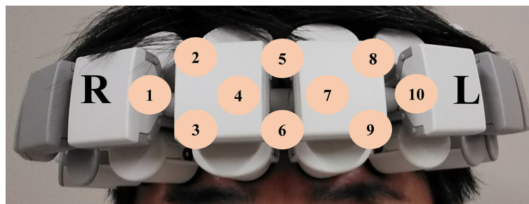
Fig. 1. Placement of NIRS probes on the prefrontal cortex.
