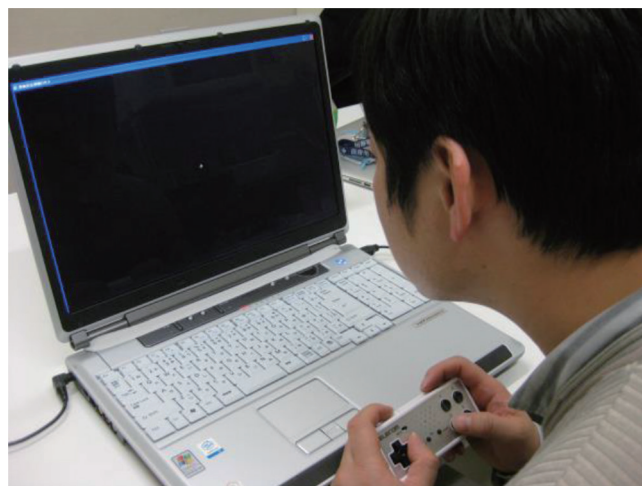
Fig. 2. Visual Field with Inhibitory Tasks (VFIT) setup. VFIT software is used to assess the UFOV. Subject sits on the front of PC monitor. They need to push the button for correct reaction.
