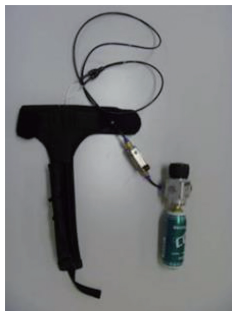
Fig. 2. The PAM used in this study is the curved type pneumatic rubber artificial muscle.
