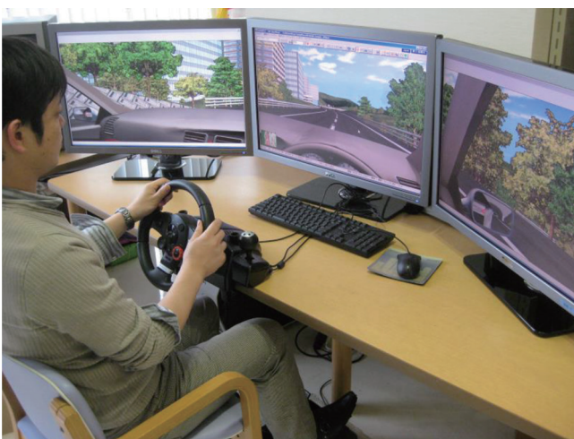
Fig. 4. Driving simulator. UC-win/ROAD software version 3.4 (FORUM8 Co., Ltd). This simulator can reflect the virtual road on three computer screens. But this software is not similar enough to a car to assess steering.
